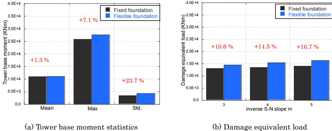
Figure 11: Statistics of tower base moment and damage equivalent load in fixed and flexible foundation
