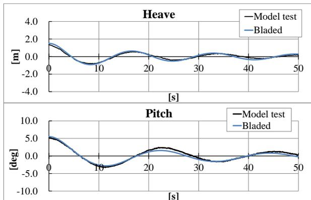
Figure 3. Comparison of the experimental and simulated free-decay motions of heave and pitch
