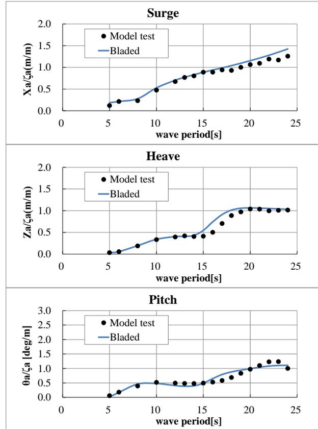
Figure 4. Comparison of the experimental and simulated RAOs of surge, heave and pitch of floater
