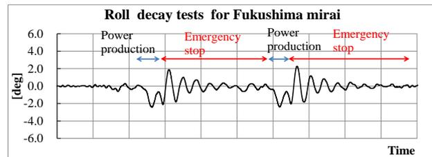
Figure 5. Time series of the rolling decay tests
