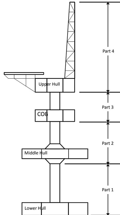
Fig. 13. Block division of offshore substation
