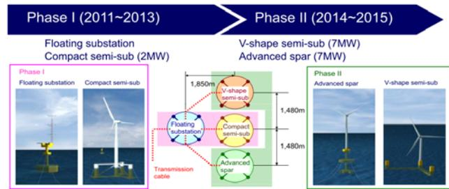
Fig. 2. Overview of Fukushima FORWARD and FOWT.
