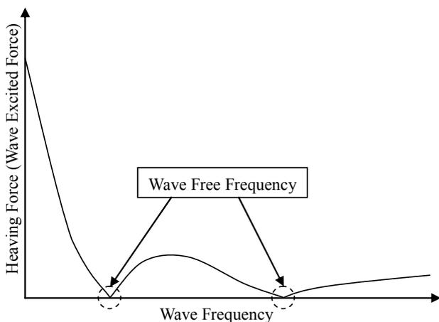
Fig. 8. 2 point wave free frequency
