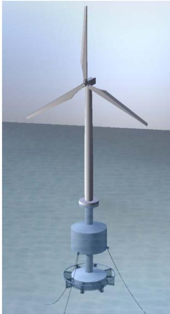
Fig. 3. Advanced spar wind turbine
