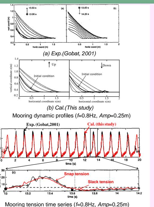
Mooring tension time series (f=0.8Hz, Amp=0.25m)
