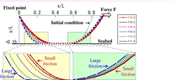
Profiles of horizontally dragged cable with different seabed friction factors
