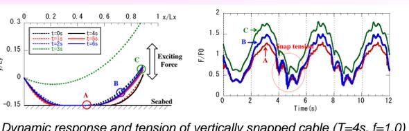
Dynamic response and tension of vertically snapped cable (T=4s, f=1.0)
